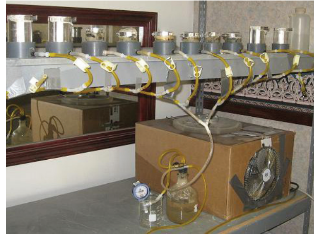
A vacuum is applied to the group of saturated samples in a parallel configuration.
