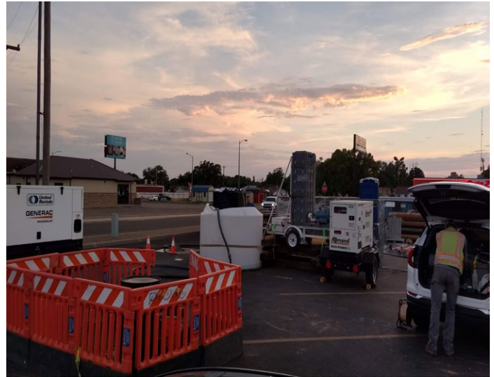
Testing was performed to characterize aquifer parameters, with extracted groundwater treated with an air stripper and discharged to the City of Clovis sanitary sewer
